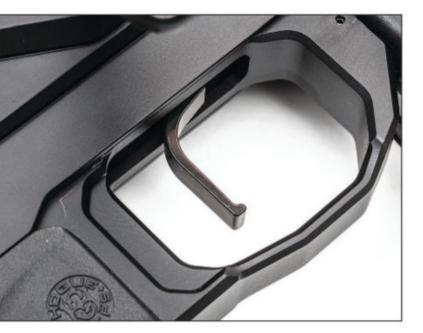
**TOP:** The MPR's flat-faced trigger lends itself to a precise rearward press, keeping the gun on target.
